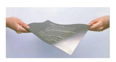
The Flex Suppressor was specially developed to absorb radiation noise from components. The sheets are typically installed in the shielding between two PCBs or directly on the radiation-emitting components. Installation is very easy because of the flexibility of the material and the self-adhesive film on the reverse side.
